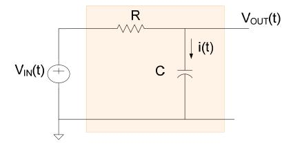
$$\tilde{V}_{OUT}(t) = \left[ V_{M} \frac{\sin \gamma}{(RC)^{2}} \left( 1 - \frac{\omega RC}{\tan \gamma} \right) e^{-t/RC} \right] + \left[ V_{M} \left( \frac{1}{\sqrt{1 + (\omega RC)^{2}}} \right) \sin(\omega t + \gamma - \tan^{-1}(\omega RC)) \right]$$
