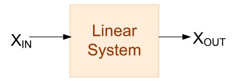
The frequency dependent gain of a linear circuit or system is often termed the transfer function
